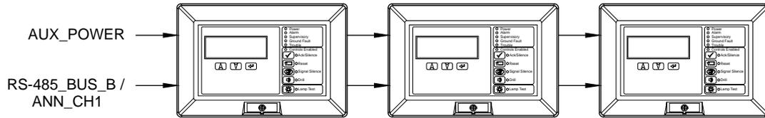
**Figure 6: Typical redundant Class B wiring**
