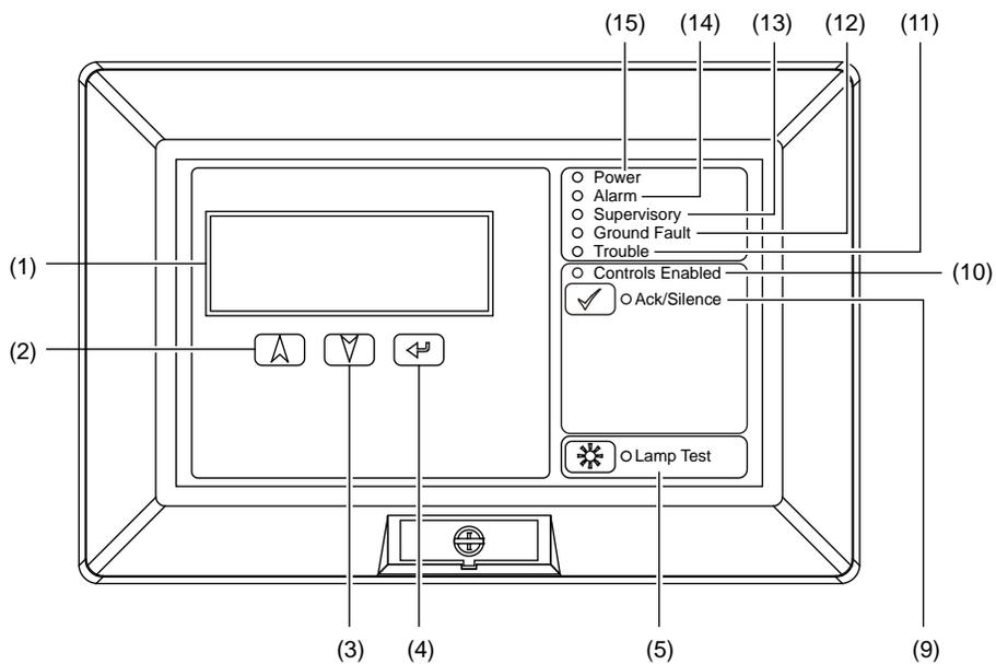
**Table 6: Controls and indicators for LCD remote annunciators (with and without common controls)**
