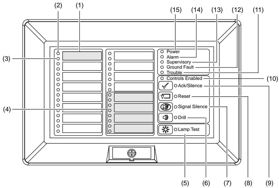
Figure 13: Controls and indicators for the K-RLED24 and K-RLED24R
