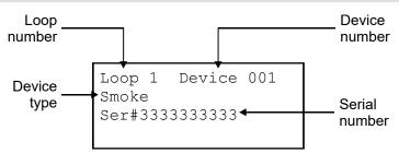
Figure 51: Internal event (panel and loop events) details display screen
