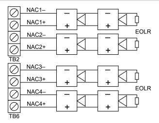
Figure 13: VS4 panel Class A NAC wiring
