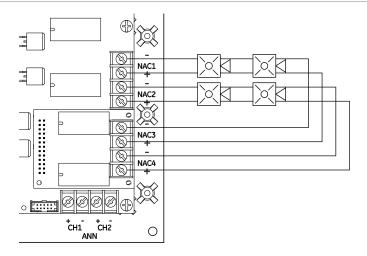
Figure 36: SA-CLA Redundant Class B remote annunciator circuit
