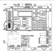
Figure 27: Auxiliary/smoke power output terminals
