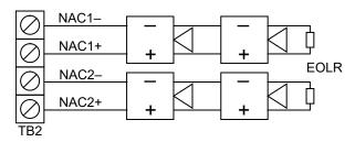
Figure 12: VS4 panel Class B NAC wiring
