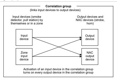
A correlation group can contain any combination of input devices, output devices, NACs, events, and zones. Input devices, output devices, NACs, events, and zones can be assigned to more than one correlation group. There are 199 available correlation groups.
