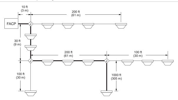
Table 50: Longest allowable circuit path with zero UM or MABs configured for two-wire smoke detectors
