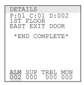
The Details display screen provides the device address and, if programmed, the location description of the device that generated the selected event message. If the selected event message were for a zone, the Details display screen would show which devices in the zone were activated.
